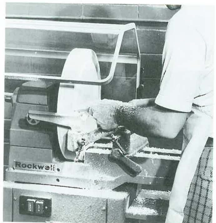
Figure 27-45. Both the face and edge can be turned without having to reposition a right angle tool rest.
