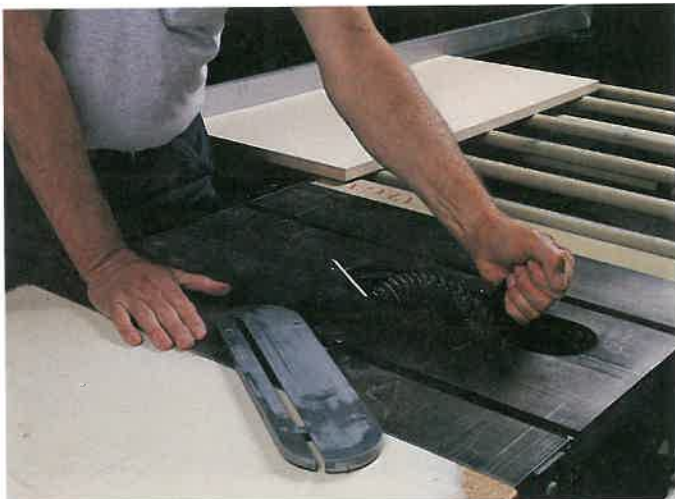
Figure 21-5. To remove the arbor nut, pull the wrench from in front of the machine. (Chuck Davis Cabinets)
