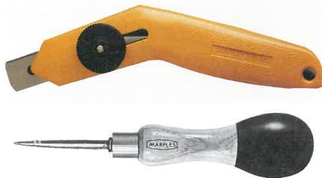
Figure 20-2. Knives and scratch awls make precise marks. A variety of styles are used. (Stanley Tools, Record Ridgway Tools, Brookstone)
