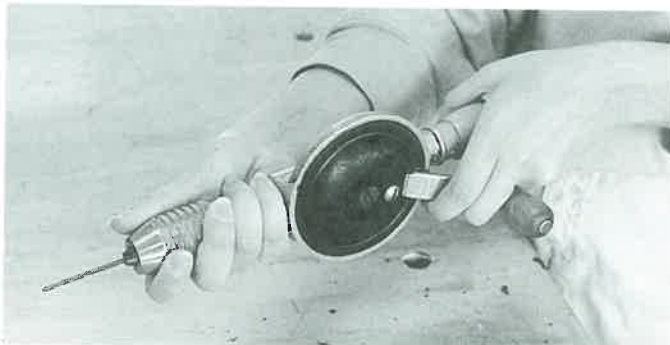
Figure 25-33. For both a brace and hand drill, install the bit and tighten the chuck by hand.
