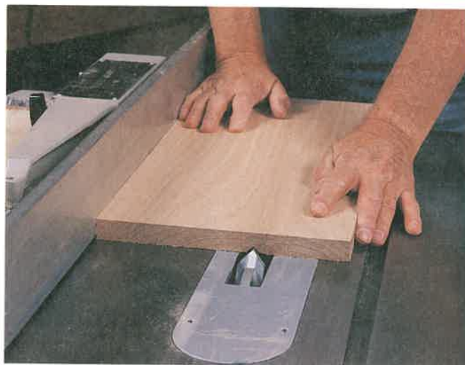
Figure 26-35. Shaping a face on the table saw. Guards removed to show operation. ( Chuck Davis Cabinets )
