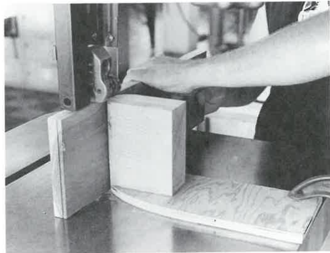
Figure 21-47. Resawing on the band saw is a one-pass operation. A—Hold material firmly against the auxiliary fence on a resaw band saw. ( Chuck Davis Cabinets ) B—Hold the material against a rounded auxiliary fence on other band saws.
