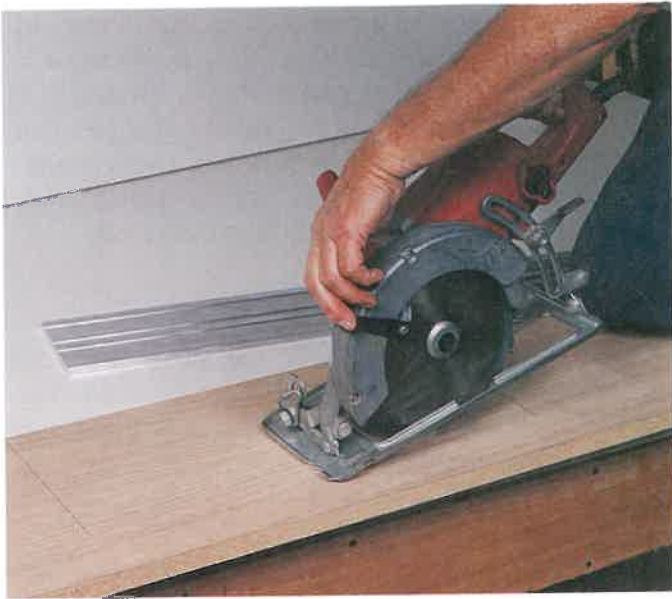
Figure 22-19. Plunge cutting with a circular saw. (Chuck Davis Cabinets)
