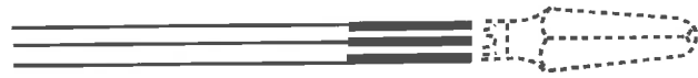
Figure 25-4. Auger bit shanks have a tang fit in a brace. The tang can be sawed off so the bit can be used in power drills. (Irwin)
