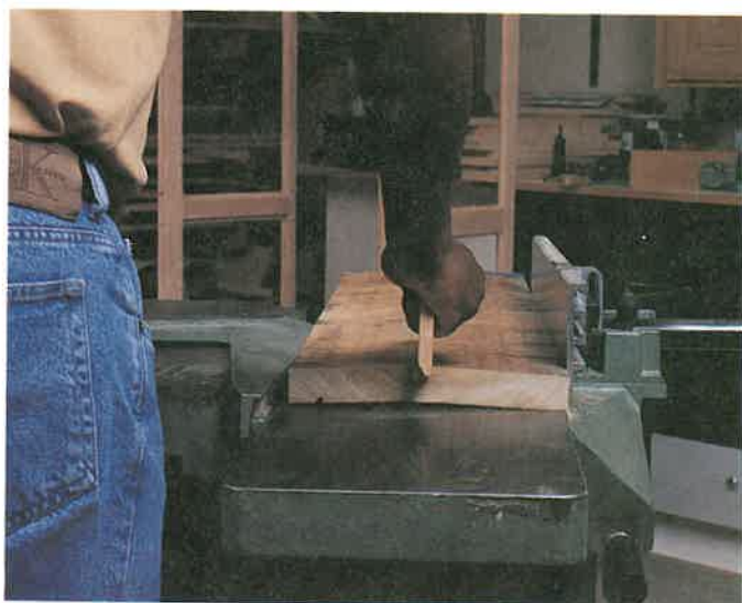
Figure 23-6. The concave side of a cupped face should be placed down. ( Chuck Davis Cabinets )
