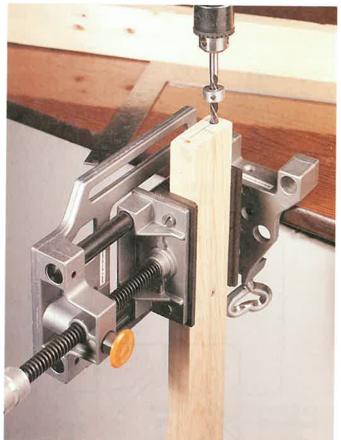
Figure 28-25. This vise holds stock in a vertical position. ( The Fine Tool Shops )
