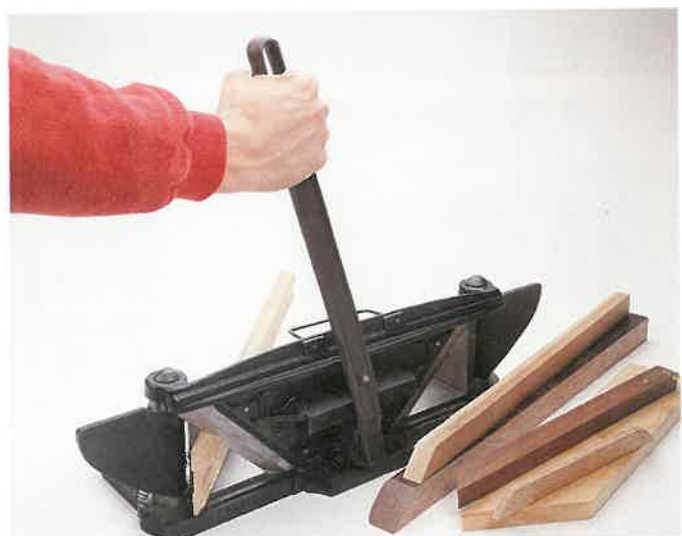
Figure 28-27. The miter trimmer shears perfect miters on molding. (The Fine Tool Shops)
