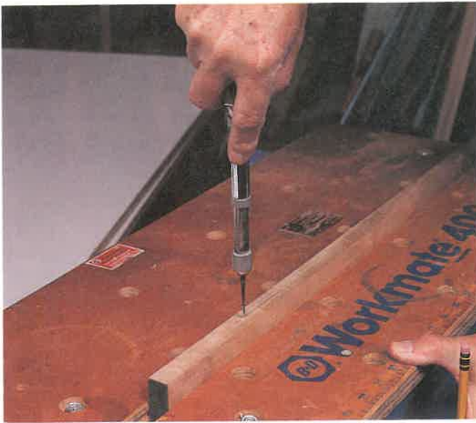
Figure 25-13. Drill points fit in a push drill. They make holes for screws, brads, and other purposes. (Chuck Davis Cabinets)
