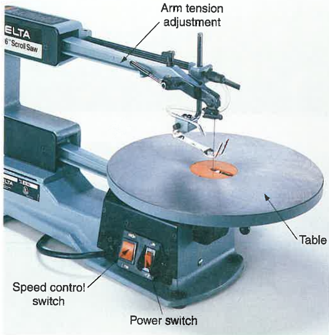
Figure 21-48. Features of a scroll saw. (Delta International Machinery Corp.)
