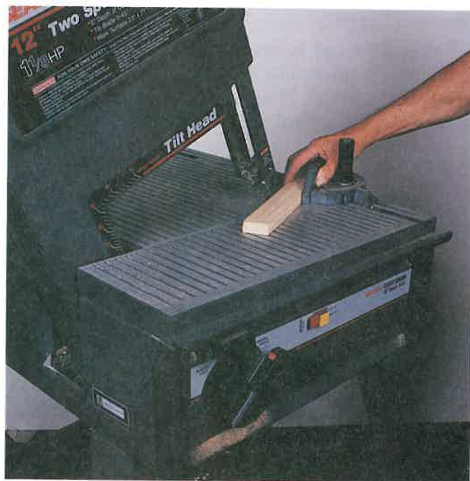
Figure 21-43. Adjust the table angle according to the tilt scale. (Delta International Machinery Corp.)
