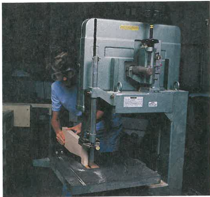
Figure 21-45. Stack material when sawing duplicate workpieces.
