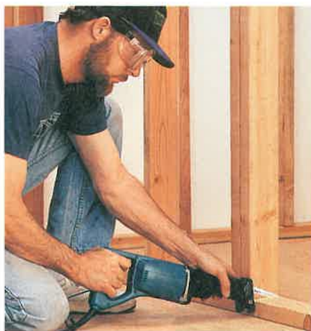
Figure 18-22. Beware of motions that can cause injury. A—Rotary. (Makita U.S.A., Inc.) B—Reciprocating. (Makita U.S.A., Inc.) C—Straight-line. (Delta International Machinery Corp.)
