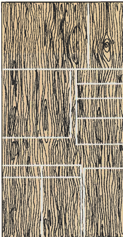
Figure 19-6. Lay out doors and drawer fronts next to each other so the grain pattern matches.
