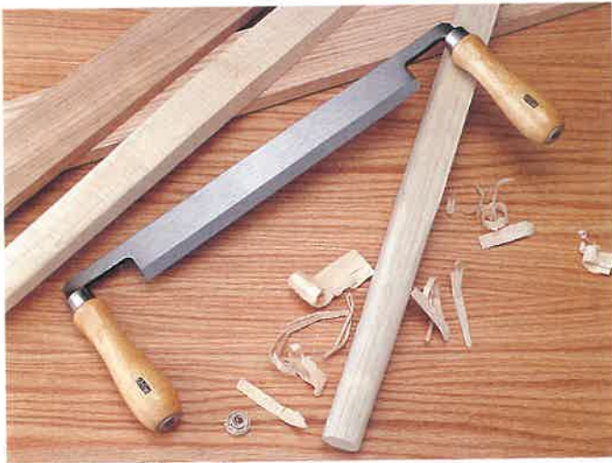
Figure 26-62. A draw knife shapes table legs quickly. ( American Machine and Tool Co. )
