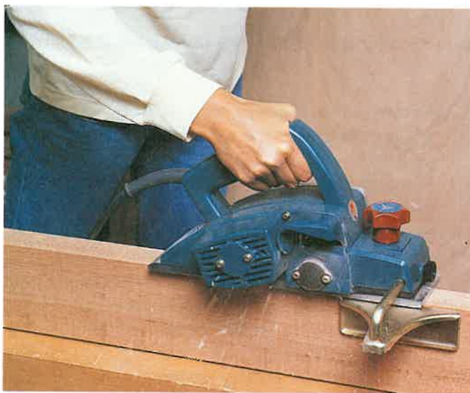
Figure 24-18. Portable power planes are useful for on-site architectural woodwork. ( Makita U.S.A., Inc. )
