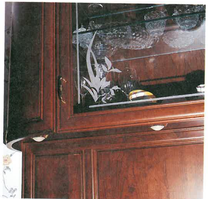
Figure 25-48. Installing low voltage halogen light. A—Boring 58 mm diameter blind hole to receive the light fixture. B—Boring hole for installation of wire. C—Assembled cabinet ready for finishing. Install light and wire before installation of cabinet. D—A completed low voltage light installation. ( Chuck Davis Cabinets )
