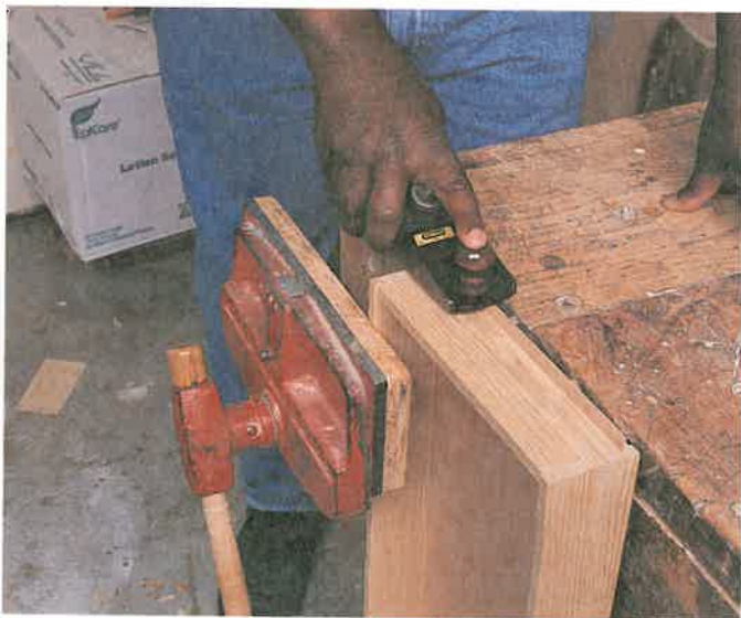
Figure 24-8. Hold a block plane in the palm of your hand.
