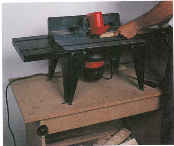
Figure 26-53. A—Mounting a router under a commercial router table. B—The router is then used like a shaper.
