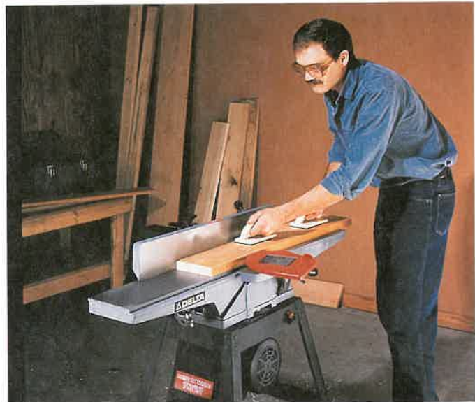
Figure 23-1. Surface lumber square on jointers and planers. (Delta International Machinery Corp.)
