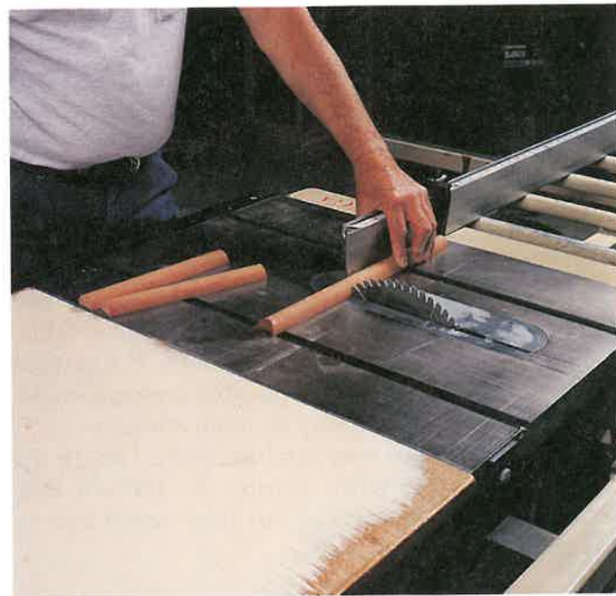
Figure 21-16. A—Stop block next to the rip fence determines the length of parts cut to duplicate lengths. B—Add the desired length of the parts to the thickness of the stop block and set the rip fence scale to the total. Guards are removed to show these procedures. (Chuck Davis Cabinets)
