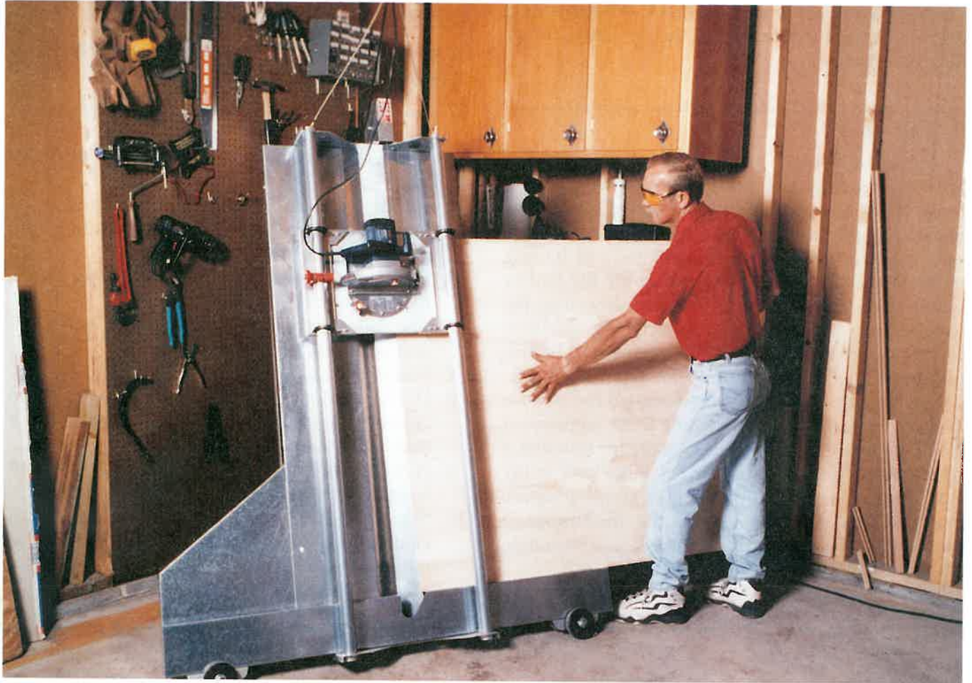
This vertical panel saw is designed to let one person cut full-sized sheets quickly, safely, and accurately. ( Panel Pro )
