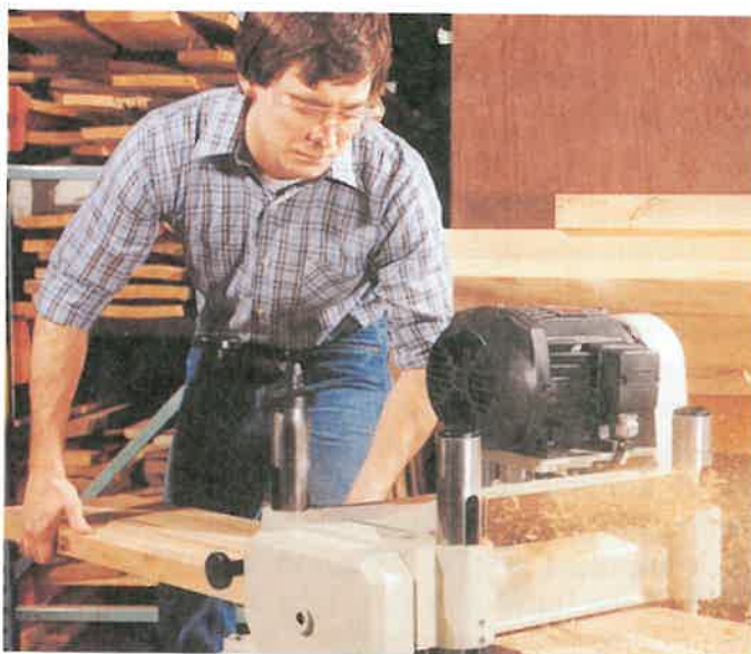
Figure 18-2. Notice how this operator is standing to one side while operating this stationary planer. ( Delta International Machinery Corp. )
