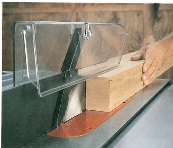
Figure 21-3. This blade guard is mounted to the saw trunnion under the table. (Delta International Machinery Corp.)
