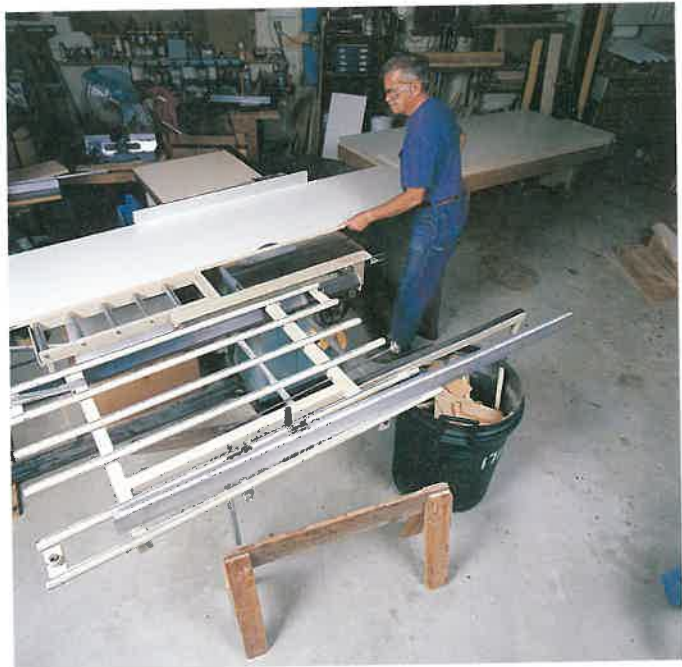
Figure 28-1. Table attachments make saw operations easier, safer, and more accurate. This table saw has the manufacturer's rip fence accessory. Aftermarket accessories are the sliding table and roller outfeed table.
