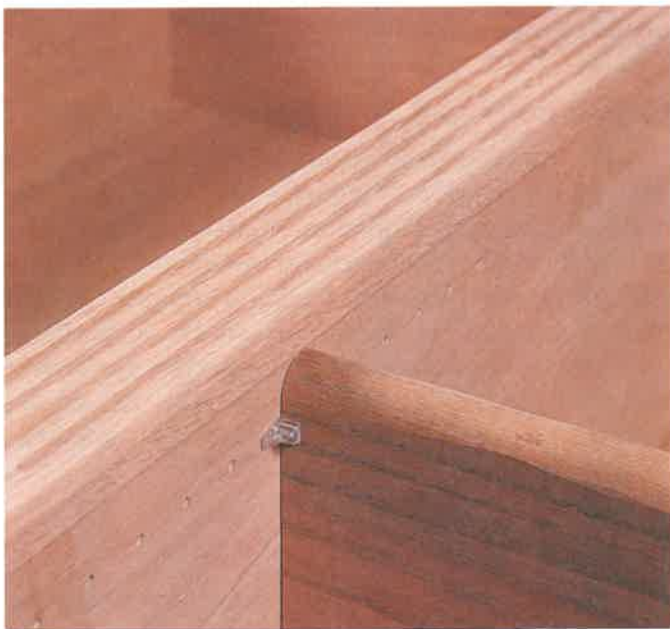
Figure 17-44. Height adjustments are limited by the number and spacing of holes. The distances between these holes are 32 mm on center. (Chuck Davis Cabinets)
