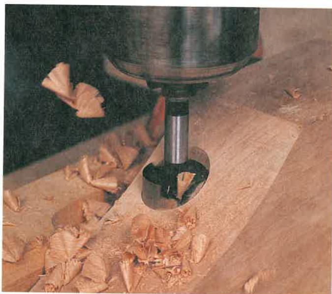
Figure 25-10. A—Forstner bits drill flat bottomed holes. B—Because its circumference guides the bit, you can bore at any angle. Clamp the workpiece securely. (Chuck Davis Cabinets)
