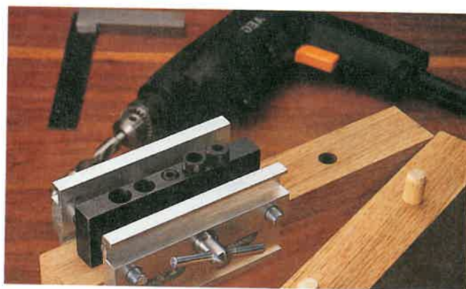
Figure 28-14. Doweling jig centers the drill bit on the edge of material. (The Fine Tool Shops)
