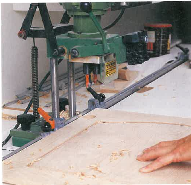
Figure 25-49. Boring blind holes for insertion of Euro-style concealed hinges. ( Chuck Davis Cabinets )
