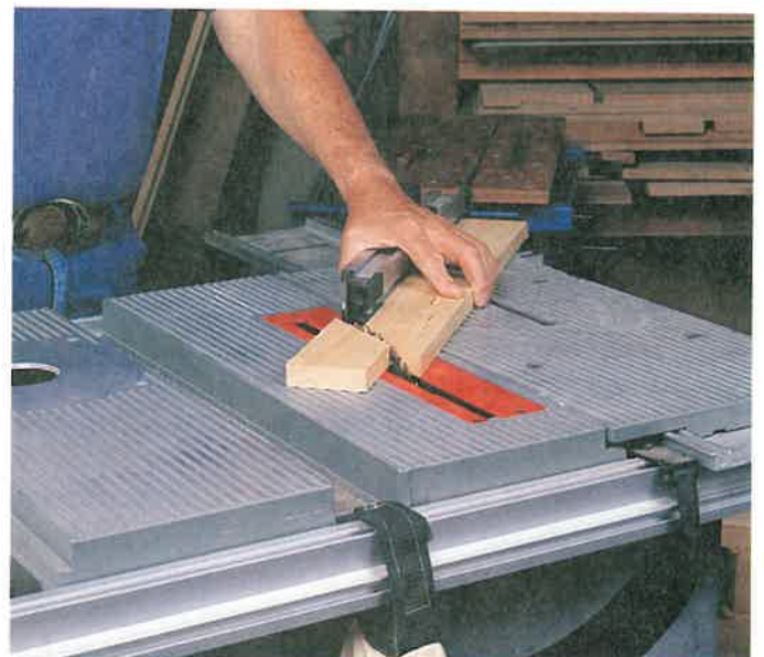
Figure 21-19. Sawing a miter. The guard has been removed to show the operation. (Chuck Davis Cabinets)
