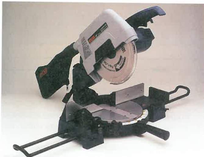
Figure 22-22. The sliding compound miter saw provides greater crosscut capacity. (Ryobi America, Inc.)
