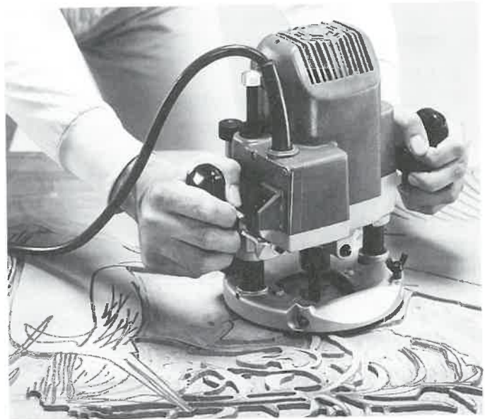
Figure 26-48. Work on carving may begin with routing out excess material. (Makita U.S.A., Inc.)
