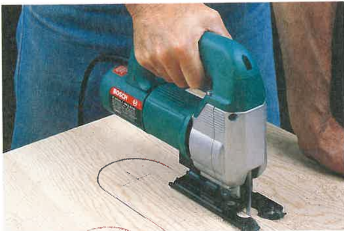
Figure 22-1. Portable power tools, such as this saber saw, are often an excellent alternative to stationary power tools. (Robert Bosch Power Tool Corp.)
