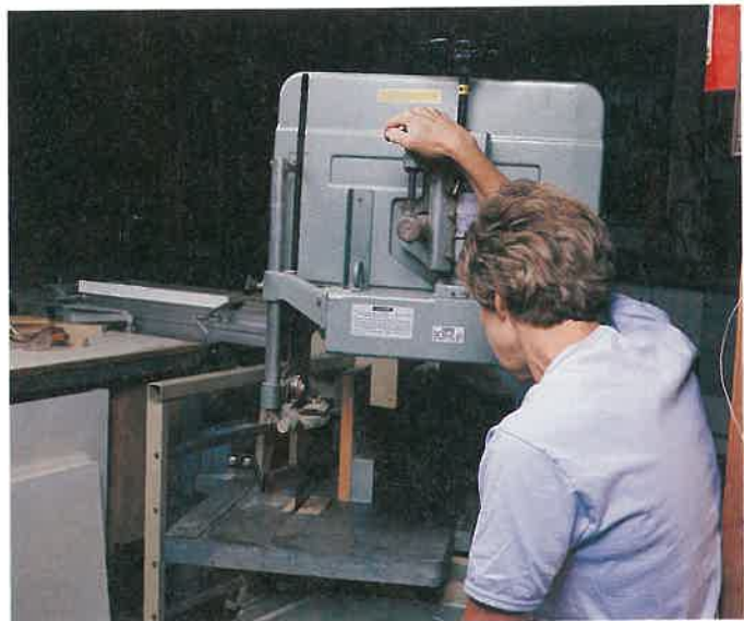
Figure 21-38. Tracking adjustment is found on the back of the machine behind the upper wheel. (Chuck Davis Cabinets)
