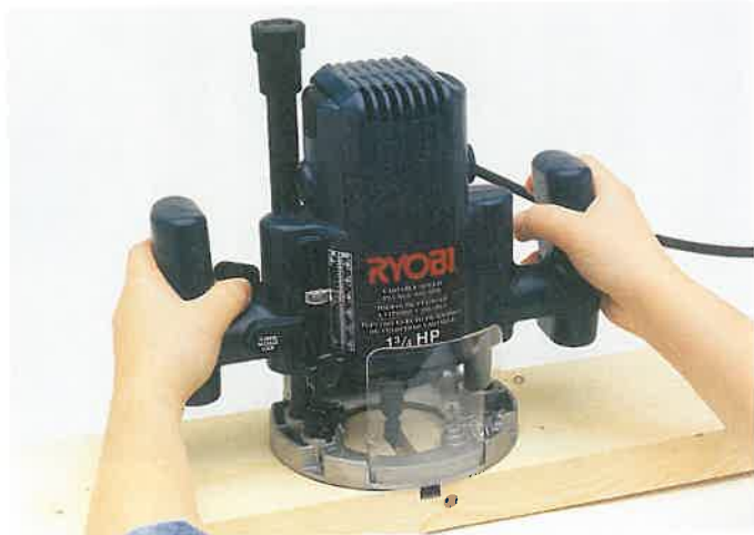
Figure 26-41 Plunge router motor moves up and down on spring-loaded posts. (Ryobi America Corp.)
