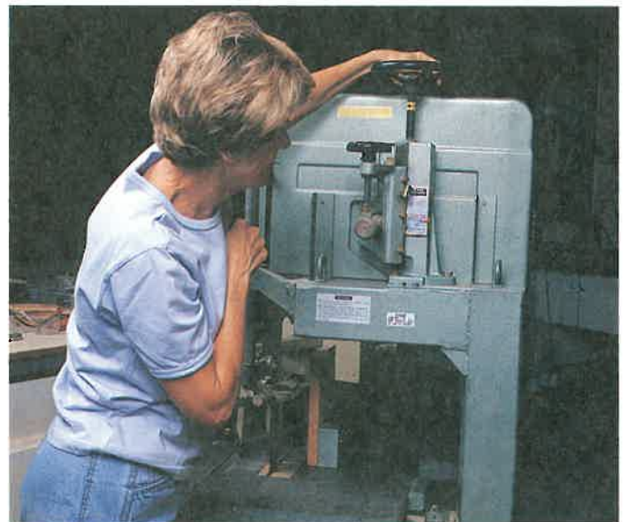
Figure 21-36. A—Remove or swing aside guards to gain access to the blade. B—Loosening blade tension. (Chuck Davis Cabinets)
