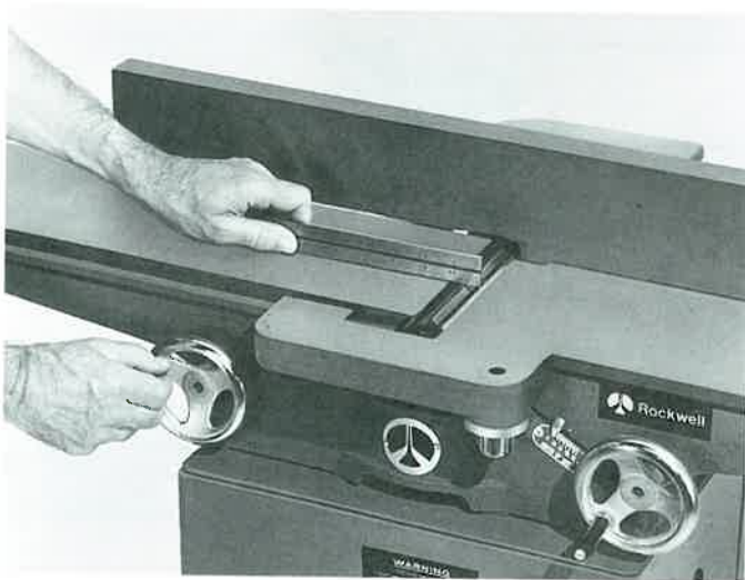
Figure 23-23. The outfeed table should be the same height as the tip of the jointer knives. (Rockwell International)
