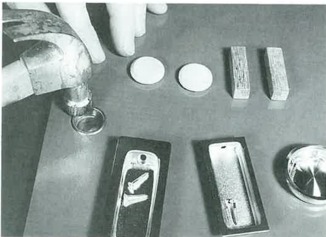
Figure 17-4. Flush mount pulls are secured by friction, glue, and/or screws. (APA - Engineered Wood Association)
