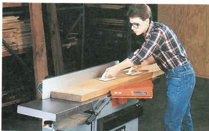
Figure 23-5. Use push sticks and push boards when jointing. Hold the board firmly against the table when face jointing. ( Delta International Machinery Corp. )
