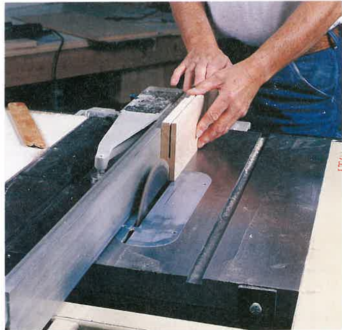
Figure 21-21. A two-pass resawing operation. A—Set the blade height just over half the material width. Keep the same surface against the fence for both passes. B—Use push sticks to feed the material as your hand nears the blade. (Chuck Davis Cabinets)
