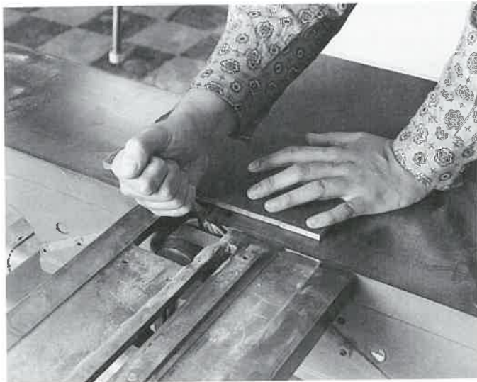
Figure 23-21. A—Loosen the gib retaining screws to remove knives. A fixture holds the cutterhead in place. (Delta International Machinery Corp.) B—Without a fixture, use hardboard to protect your hands.
