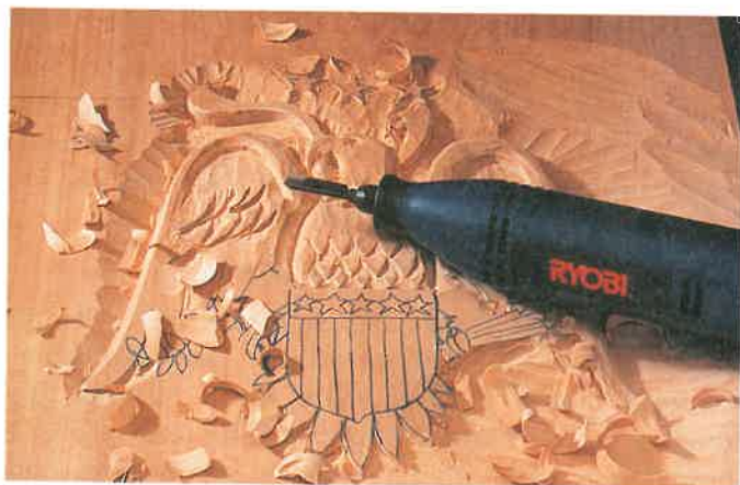
Figure 26-55. Power carving tool. (Ryobi North America, Inc.)
