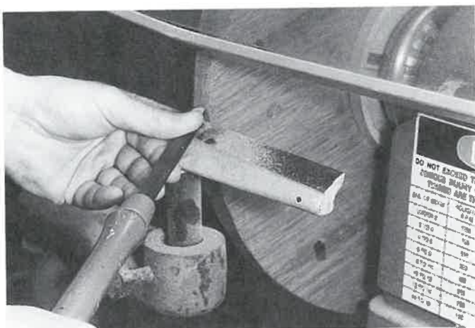
Figure 27-46. Guard slides to the outboard side of the headstock.
