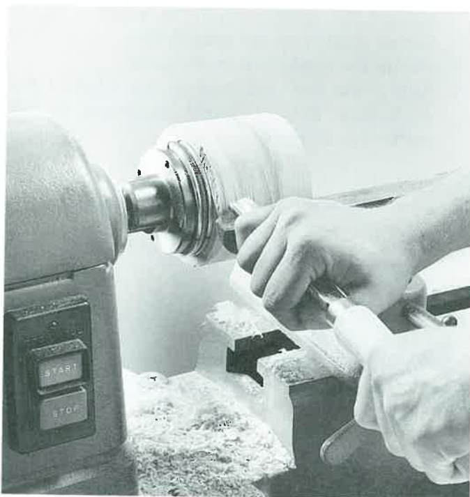
Figure 27-43. A gouge quickly turns the edge to diameter. The guard was removed to show the operation.
