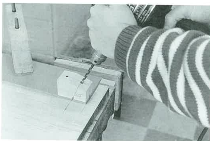
Figure 25-39. Angled holes can be accurately drilled with a jig.
