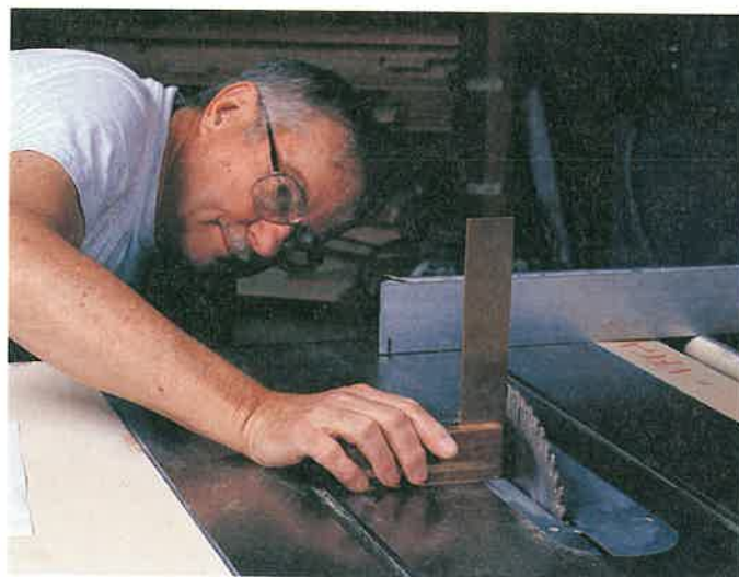
Figure 21-10. Checking to ensure the blade is at 90° to the table. Avoid placing the square on a tooth or its brazing. (Chuck Davis Cabinets)
