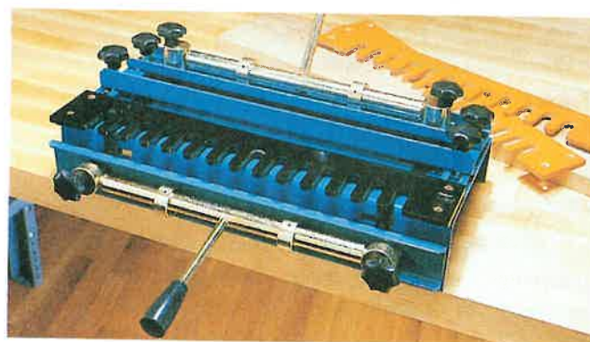
Figure 28-15. A dovetail jig allows you to cut dovetail joints with a portable router. (American Machine and Tool)
