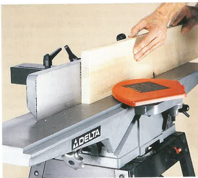
Figure 23-7. Edge-jointing. Your left hand holds the workpiece against the fence. Your right hand does the feeding. (Delta International Machinery Corp.)
