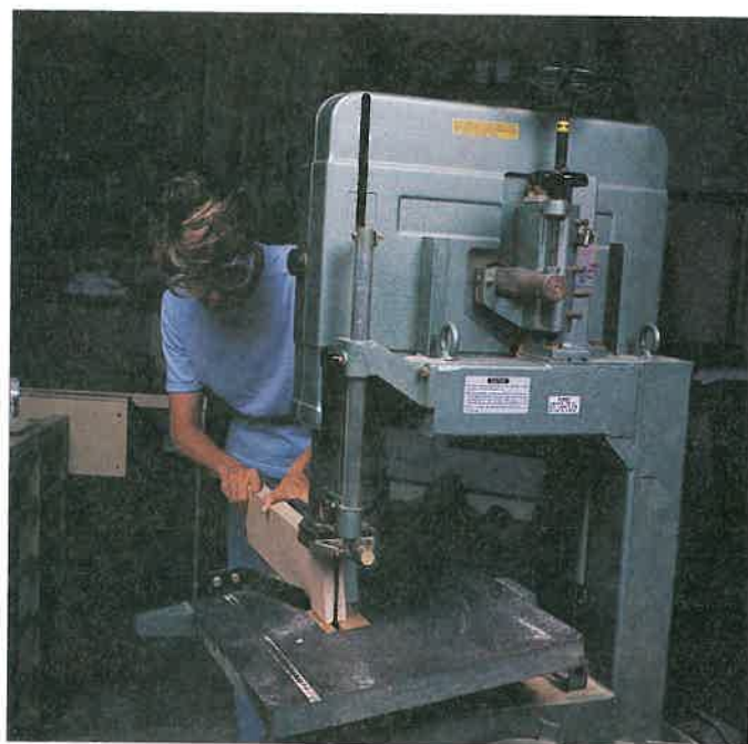
Figure 21-44. Beveling on the band saw. A—A tilting head and a miter gauge is used to produce a compound bevel. (Chuck Davis Cabinets) B—A tilting table and fence may be used for straight bevel. (Chuck Davis Cabinets)
