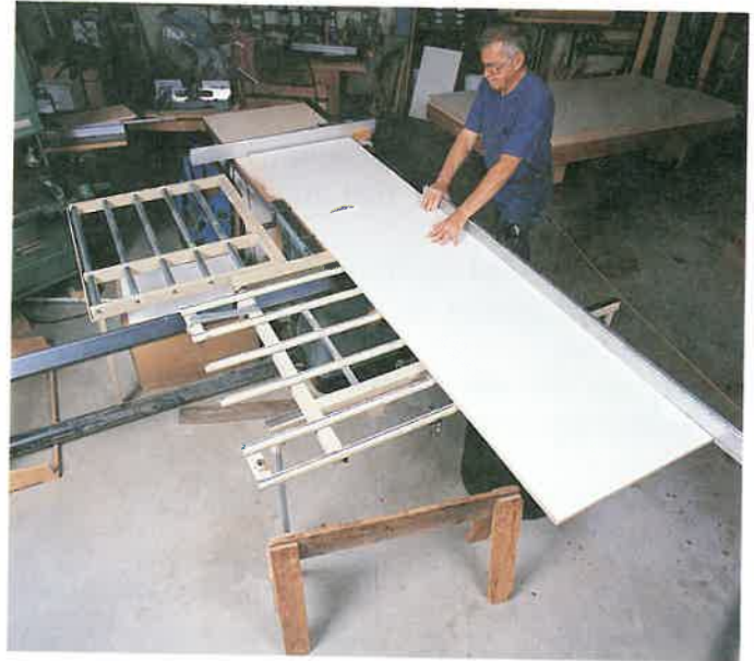
Figure 28-4. A gliding table supports longer and heavier stock for cross and miter cuts. The miter gauge features a stop and scale to 72" (1.83 m). The stop was rotated up and out of the way for this trimming operation. ( Chuck Davis Cabinets )
