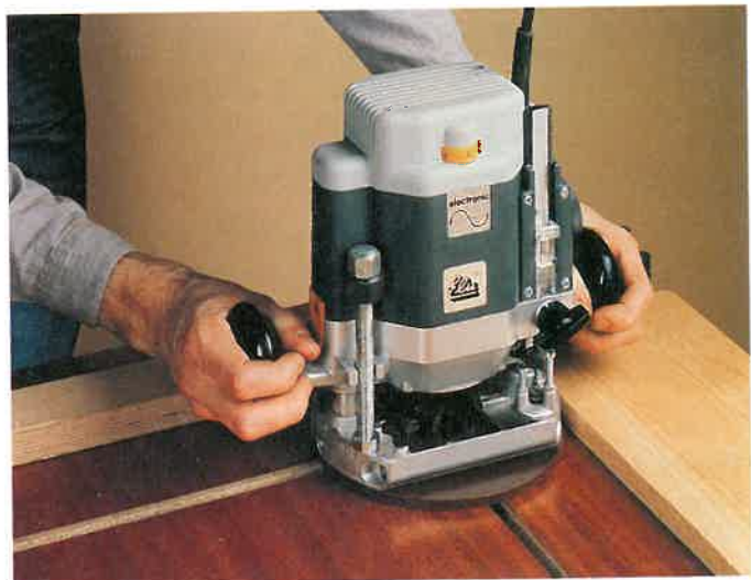
Figure 26-42. The router base rides along the straightedge for grooving this door panel. (Black & Decker)
