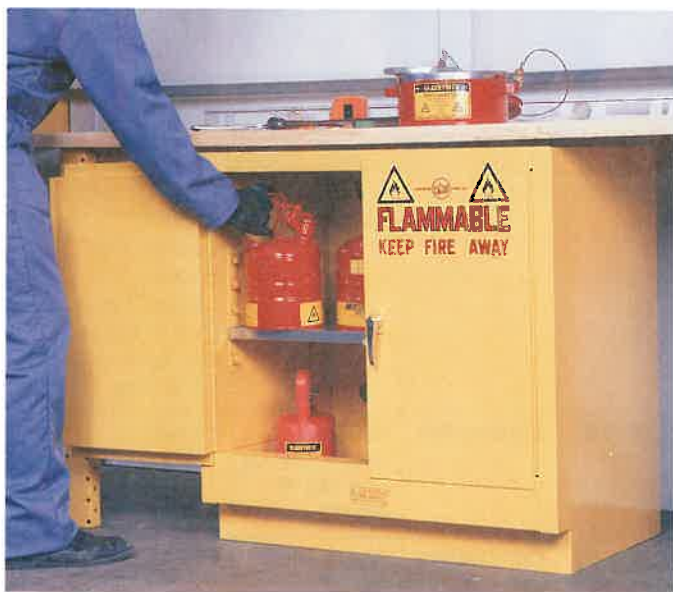
Figure 18-6. An approved safety cabinet will resist fire for a period of time. It also is watertight to retain any leaking fluids. (Justrite Manufacturing Co.)
