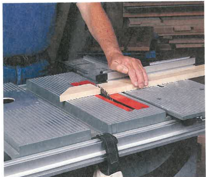
Figure 21-13. Crosscutting with the miter gauge. The guard was removed to show the operation.
