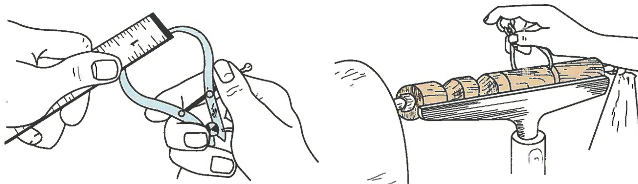
Figure 20-20. Set and use the outside caliper to check diameter measurements. (The L. S. Starrett Co.)
