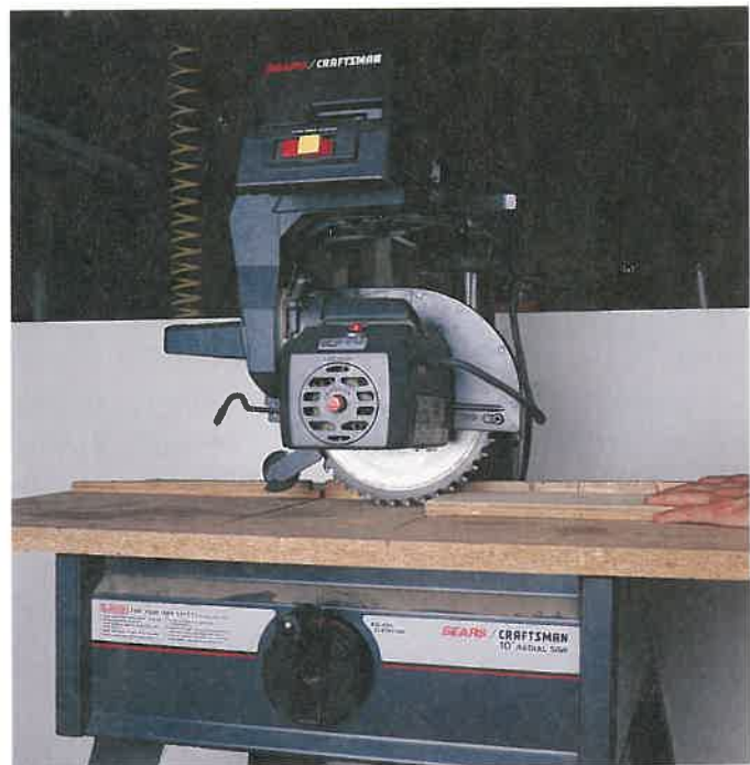
Figure 21-30. Feed material against the rotation of the blade when ripping.
