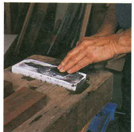
Figure 24-19. Hone a plane iron at an angle just greater than the bevel. A—Start with an 800 grit waterstone, progress to 1200 grit. B—Finish with 6000 grit. C—Then hone several strokes on the flat side of the iron using the 6000 grit waterstone. ( Chuck Davis Cabinets )
