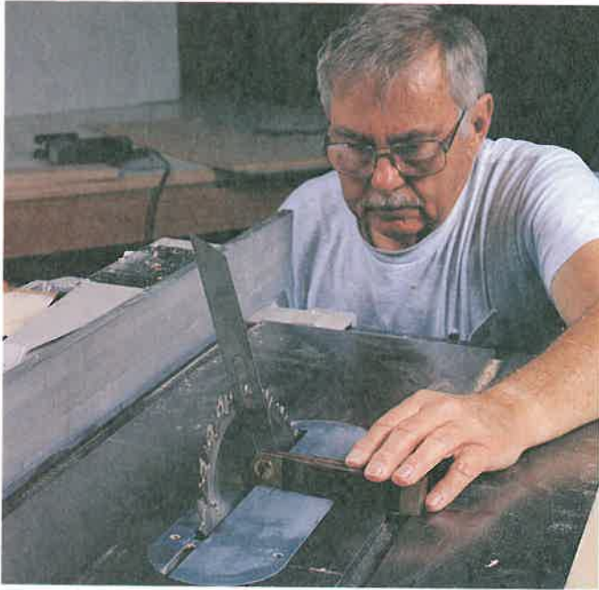
Figure 21-17. First set the T-bevel angle with a protractor and then set blade tilt. (Chuck Davis Cabinets)
