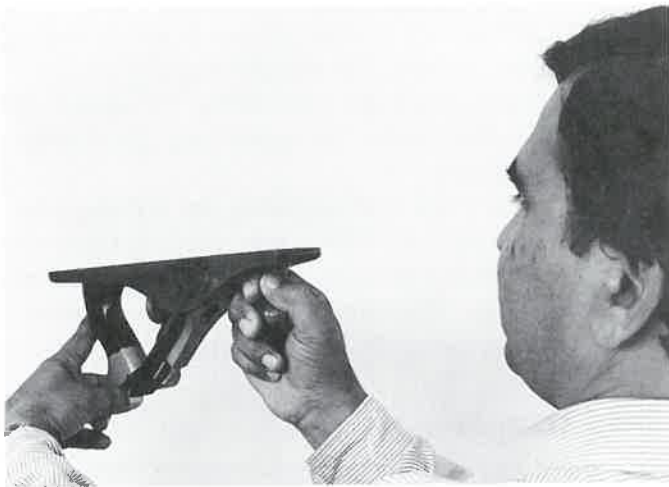
Figure 24-5. Sight down the sole to check whether the plane iron extends equally through the mouth.
