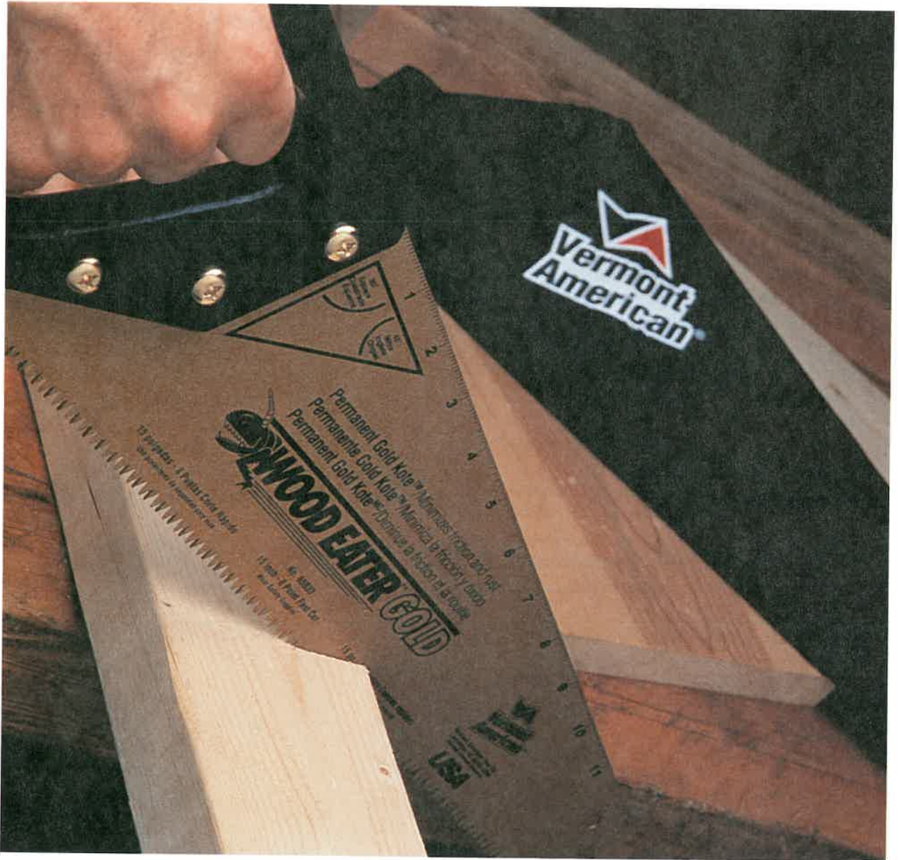
Shown is the proper technique for cutting with a handsaw. ( Vermont American )
