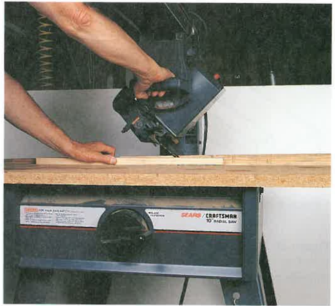
Figure 21-32. Beveling with a radial arm saw.
