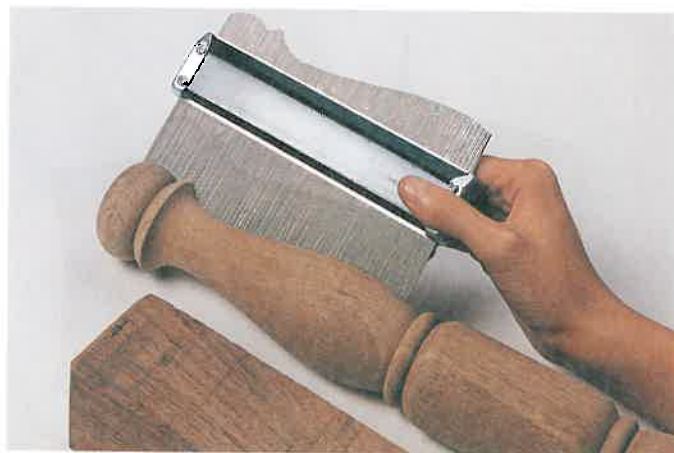
Figure 20-26. The template former conforms to the shape of the piece to be copied. ( The Fine Tool Shops )
