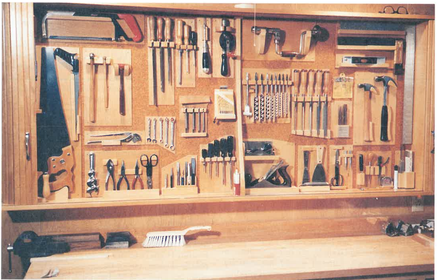
Figure 18-10. This shop has a well organized tool cabinet. After using a tool it should be returned to its proper place.
