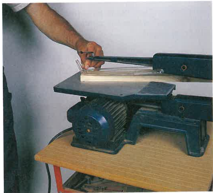
Figure 21-51. When cutting interior curves, free the top end of the blade and thread it through a predrilled hole.
