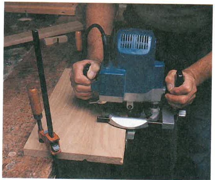
Figure 26-45. Shaping an edge using a router fence to guide the bit. (Chuck Davis Cabinets)
