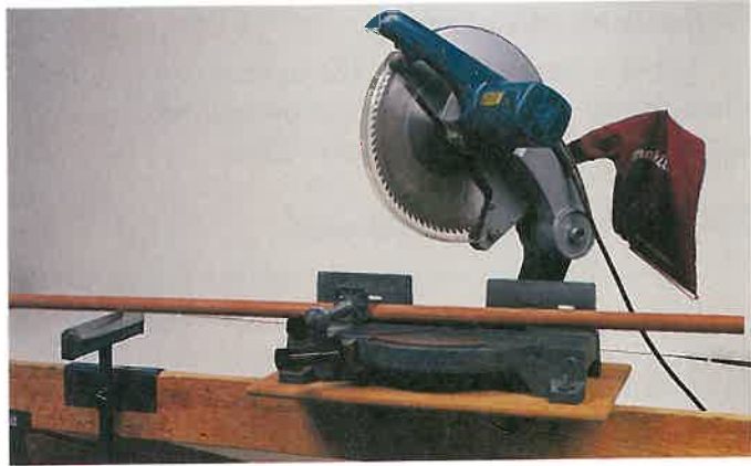
Figure 22-20. Power miter saw set to cut molding. (Chuck Davis Cabinets)
