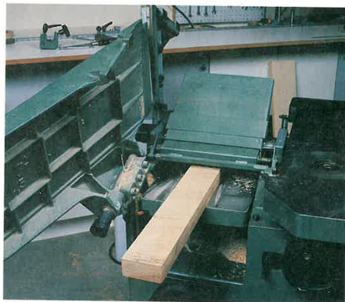
Figure 23-10. Planers surface material to thickness after jointing the first face. (Chuck Davis Cabinets)
