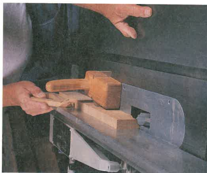
Figure 26-34. Shaping an edge on the table saw. ( Chuck Davis Cabinets )
