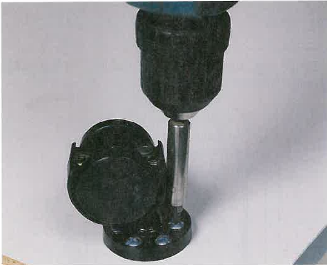
Figure 17-48. A—Casters may be pin and sleeve mounted. B—Similar casters are plate mounted. (Chuck Davis Cabinets)
