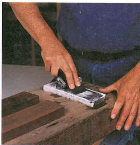
Figure 24-19. Hone a plane iron at an angle just greater than the bevel. A—Start with an 800 grit waterstone, progress to 1200 grit. B—Finish with 6000 grit. C—Then hone several strokes on the flat side of the iron using the 6000 grit waterstone. ( Chuck Davis Cabinets )
