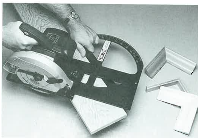
Figure 22-18. This circular saw accessory allows you to cut angles. (Matrix Enterprises)
