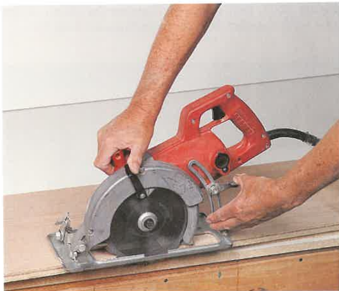
Figure 22-13. Set the blade 1/8" (3 mm) deeper than the material thickness. ( Chuck Davis Cabinets )
