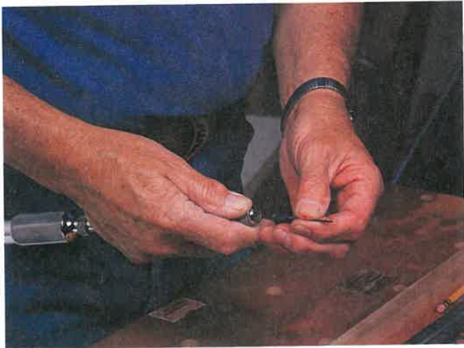
Figure 25-26. A—Push drills are very efficient for drilling small holes. B—Insert bits in the push drill by pushing the knurled chuck forward. (Chuck Davis Cabinets)
