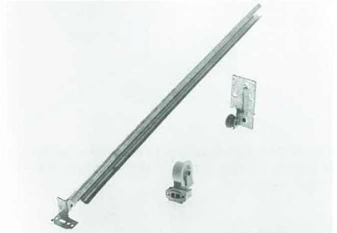
Figure 17-39. Most side mount drawer slides consist of two tracks. The forward roller, located on the cabinet track, supports the weight of the drawer. The rear roller, located on the drawer track, prevents the drawer from tipping forward when it is extended.
