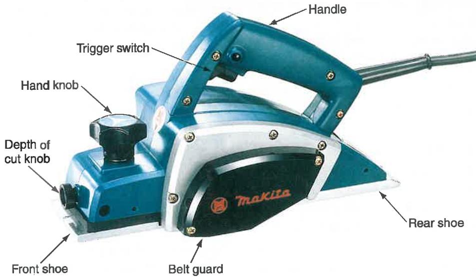
Figure 24-16. Portable power plane. This model features double-edged tungsten-carbide blades. (Makita U.S.A., Inc.)
