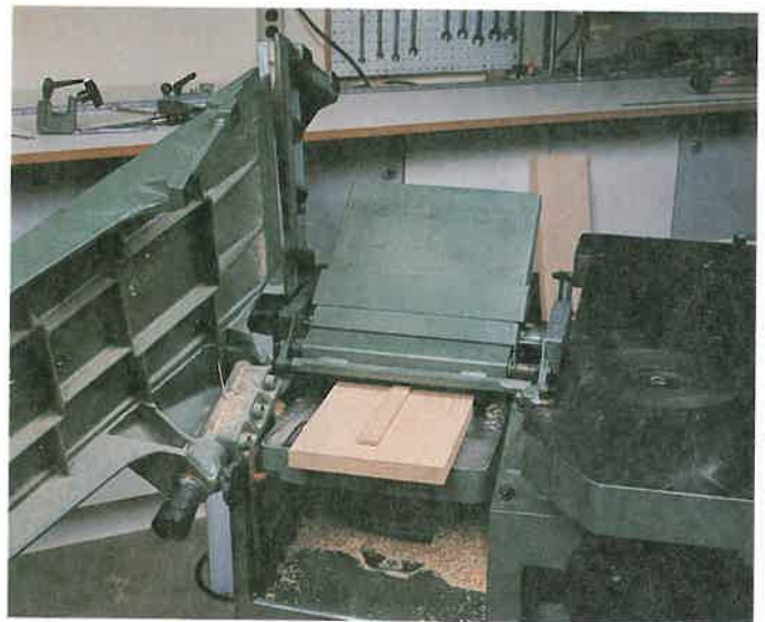
Figure 23-13. Surfacing thin material requires a backing board. (Chuck Davis Cabinets)
