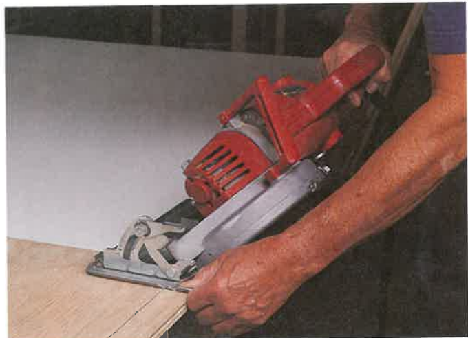
Figure 22-15. It is difficult to align with a marked line when beveling. ( Chuck Davis Cabinets )
