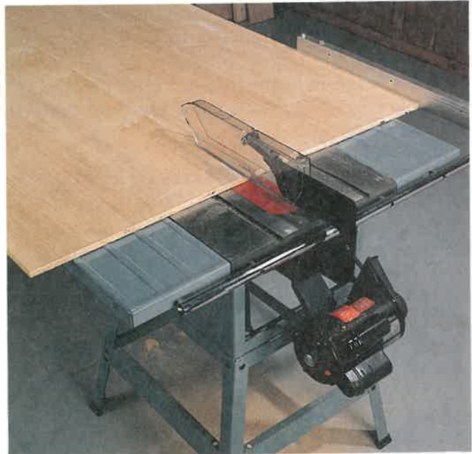
Figure 21-12. Ripping plywood. Guards are removed to show the operation. (Delta International Machinery Corp.)
