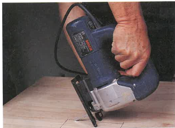
Figure 22-28. Plunge cutting with a saber saw. The tip of the blade must not bounce on the material. (Chuck Davis Cabinets)
