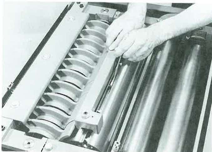
Figure 23-28. Loosen gib retaining screws to remove planer knives. ( Delta International Machinery Corp. )
