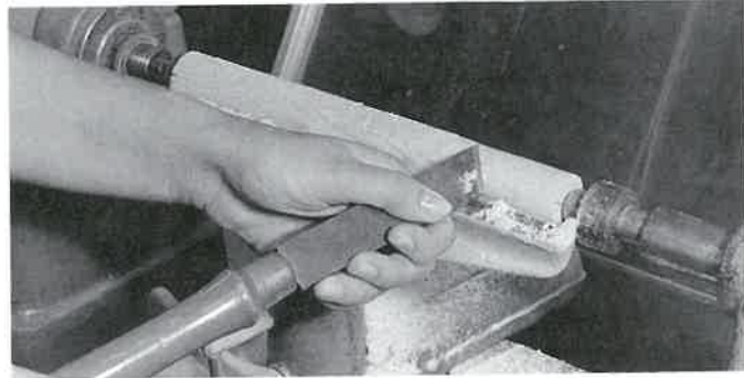
Figure 27-1. Between-center turning for making spindle products. The guard was removed to show the operation.
