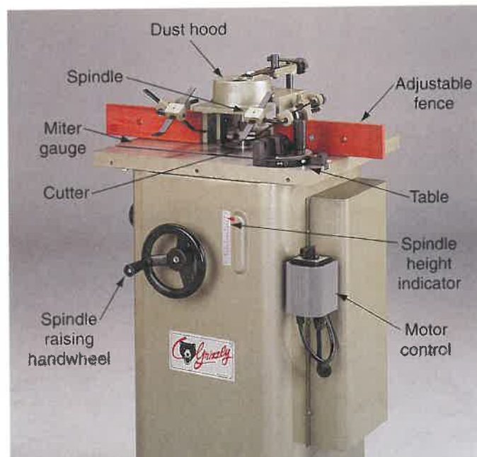
Figure 26-2. Main parts of a standard 1½ hp shaper. The fence and guard are shown in place. (Grizzly Imports, Inc.)
