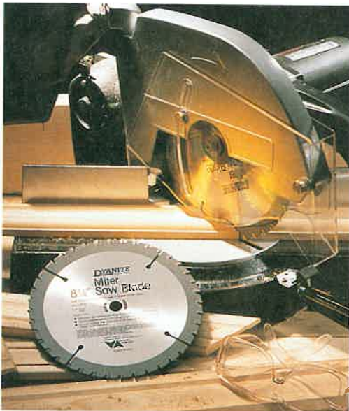
Figure 22-10. A portable power saw is a handy tool for rough-cutting lumber. (Vermont American Tool Co.)
