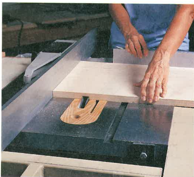
Figure 21-8. Both the rip fence and sliding table (miter gauge) are used for cuts not completely through the material. A dado cut is shown. The guard must be removed to allow this operation. (Chuck Davis Cabinets)
