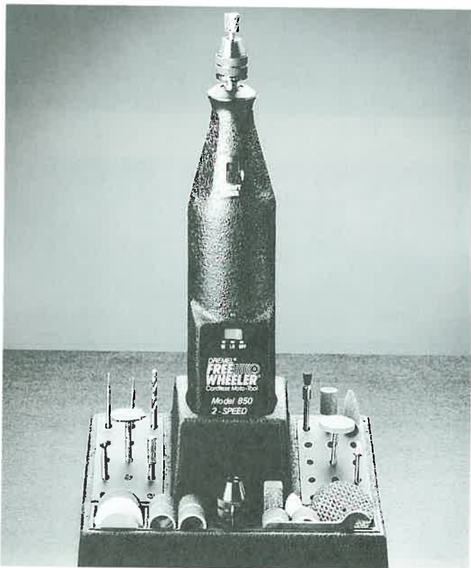
Figure 26-54. A Moto-Tool® comes with various bits. Shaping bits remove material quickly from small areas. (Dremel)
