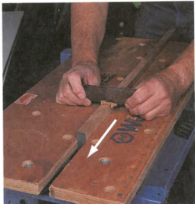
Figure 24-11. A—Cabinet scrapers are an excellent tool for smoothing the surface of parquet surfaces. ( Butler Specialty Co. ) B—Scrape with blade leaning toward the direction of cut. ( Chuck Davis Cabinets )
