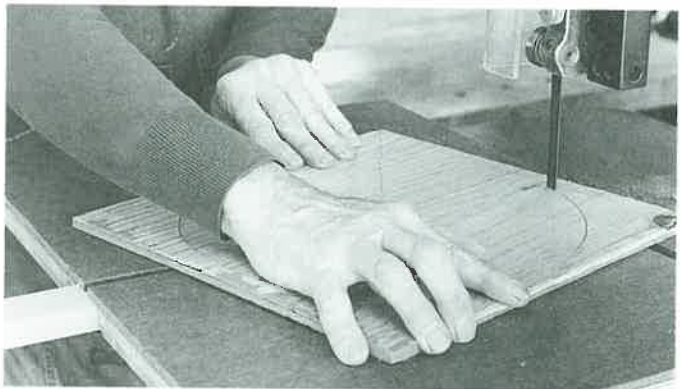
Figure 28-18. Circle cutting jig attached to the guide post of the band saw. ( Delta International Machinery Corp. )
