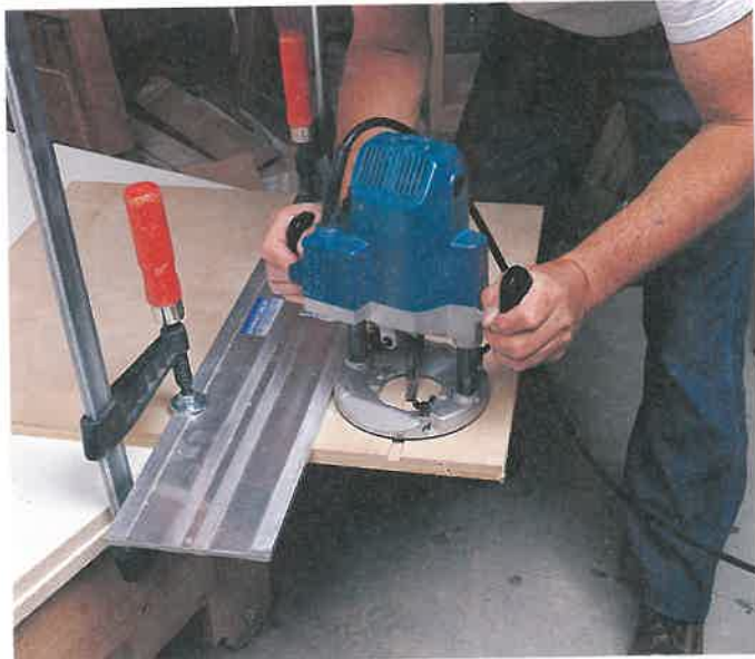
Figure 26-47. Guide the router with a straightedge to cut a dado. (Chuck Davis Cabinets)
