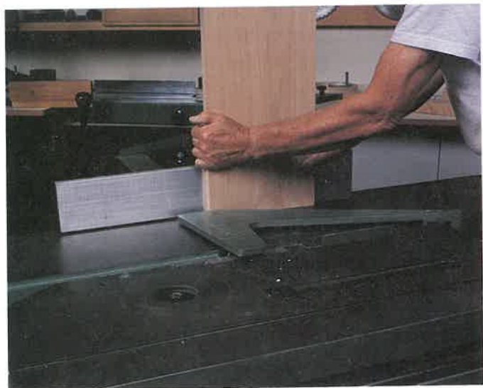
Figure 23-8. Jointing an end. A—Joint about 1" (25 mm) of an end. B—Turn the workpiece around and finish surfacing. (Chuck Davis Cabinets)
