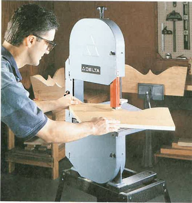
Figure 21-39. With large, curved workpieces, first cut away as much waste as possible to prevent it from hitting the machine frame. (Delta International Machinery Corp.)
