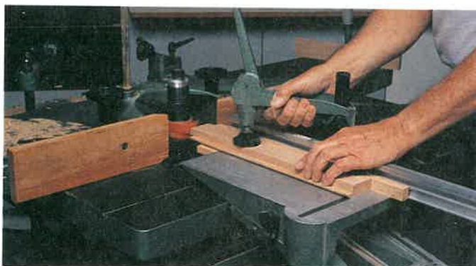
Figure 26-4. Narrow workpieces are held in a sliding table. A backer board reduces tear out. (Chuck Davis Cabinets)
