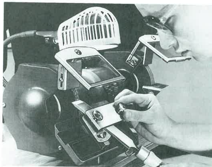
Figure 27-50. A jig allows you to precisely set the tool angle. ( Rockwell International )
