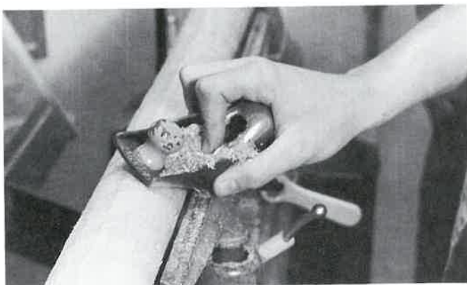
Figure 27-28. Turning a cylinder by scraping, cutting, or planing. The guard was removed to show the operation.
