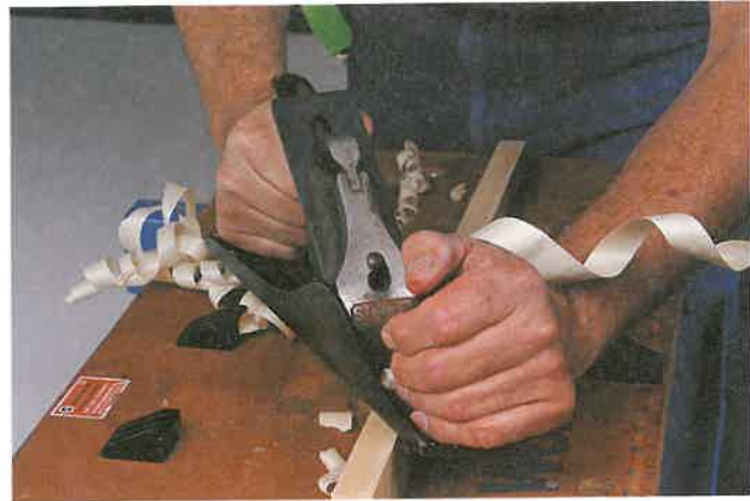
Figure 24-6. Turn the plane at an angle for easier cutting. The shavings should be thin.
