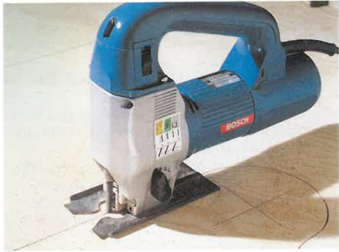
Figure 22-26. When making a series of circular cuts with the saber saw, use a line to guide the cut. (Bosch Power Tools)
