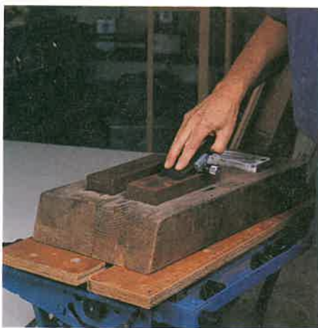
Figure 24-19. Hone a plane iron at an angle just greater than the bevel. A—Start with an 800 grit waterstone, progress to 1200 grit. B—Finish with 6000 grit. C—Then hone several strokes on the flat side of the iron using the 6000 grit waterstone. ( Chuck Davis Cabinets )
